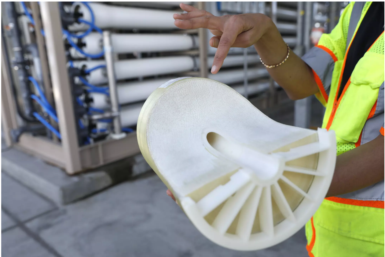
Rupam Soni, a community relations team manager, shows a cutaway of part of a reverse-osmosis treatment system during a tour of the Metropolitan Water District’s pilot water recycling facility in Carson. (Christina House/Los Angeles Times)
