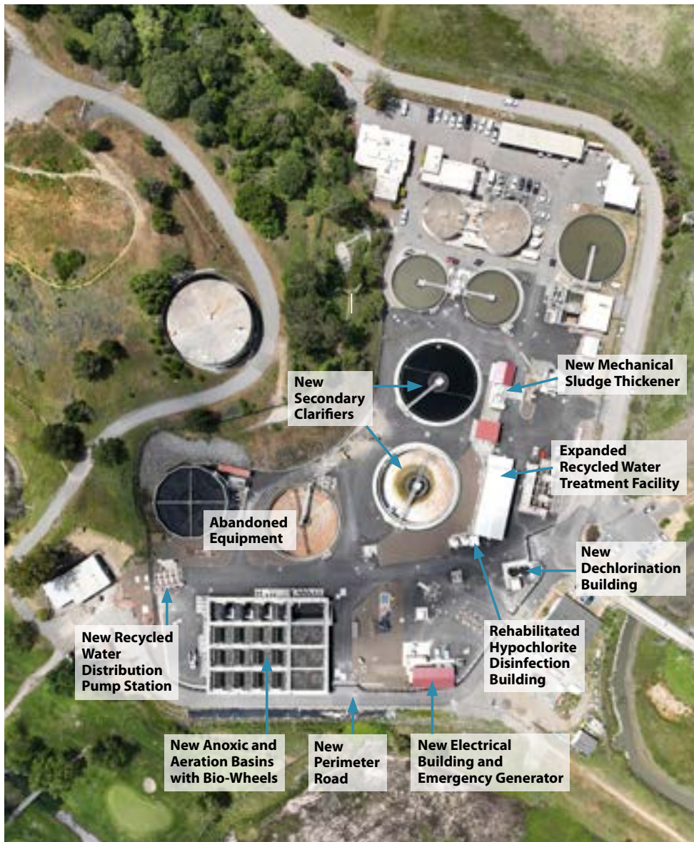
Aerial view shows key improvements/upgrades accomplished during the nearly four years of construction.
