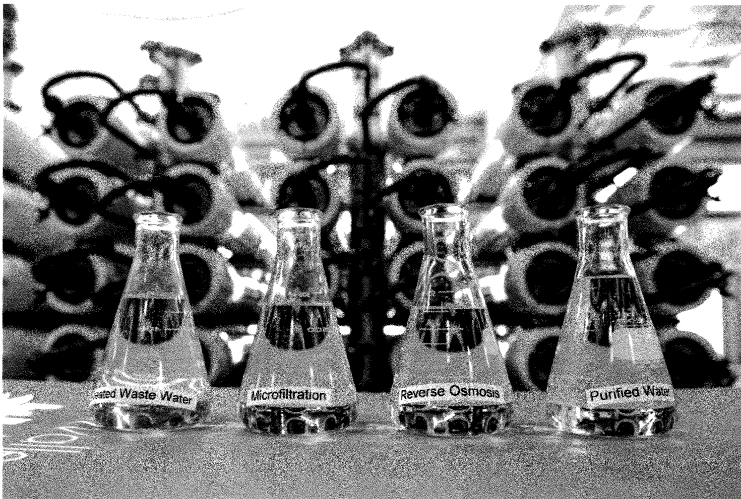
Beakers on display show results of the four steps in the water-purification process: treated wastewater, microfiltration, reverse osmosis and purified water, at the Silicon Valley Advanced Water Purification Center in San José on Sept. 23, 2021. (Beth LaBerge/KQED)
